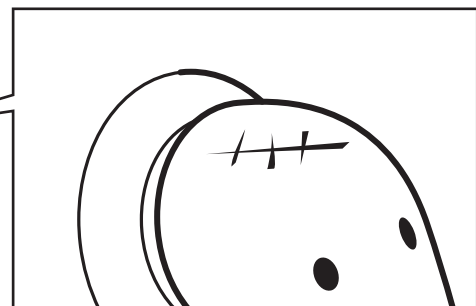
Example of scratch on plated surface
